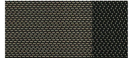
BROKEN TWILL CONSTRUCTION
